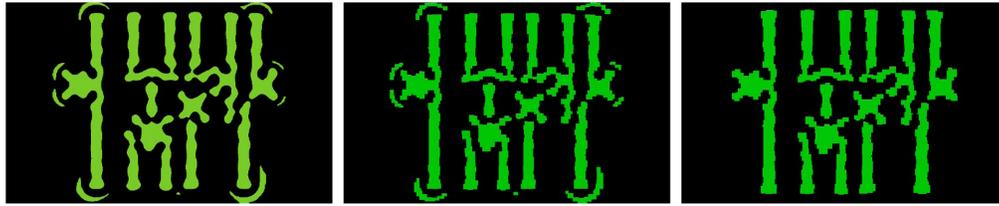
**Fig. 6** ILT mask patterns shown in the 2005 Luminescent ILT shows the curvilinear ILT mask patterns and the Manhattanized mask patterns<sup>15</sup> (source: Luminescent/Synopsys).
