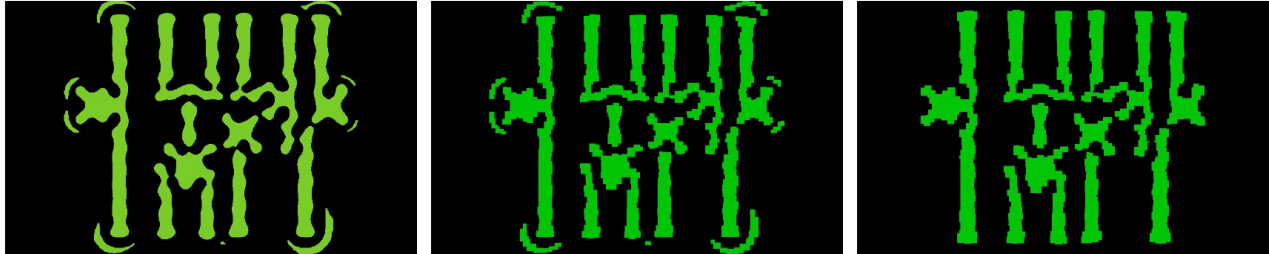
Figure 1. Mask pattern created by this first ILT solution (left). “Manhattanized” version of the same pattern (center), Manhattanized ILT mask patterns without SRAFs. (right)[1]. Source: Luminescent/Synopsys
